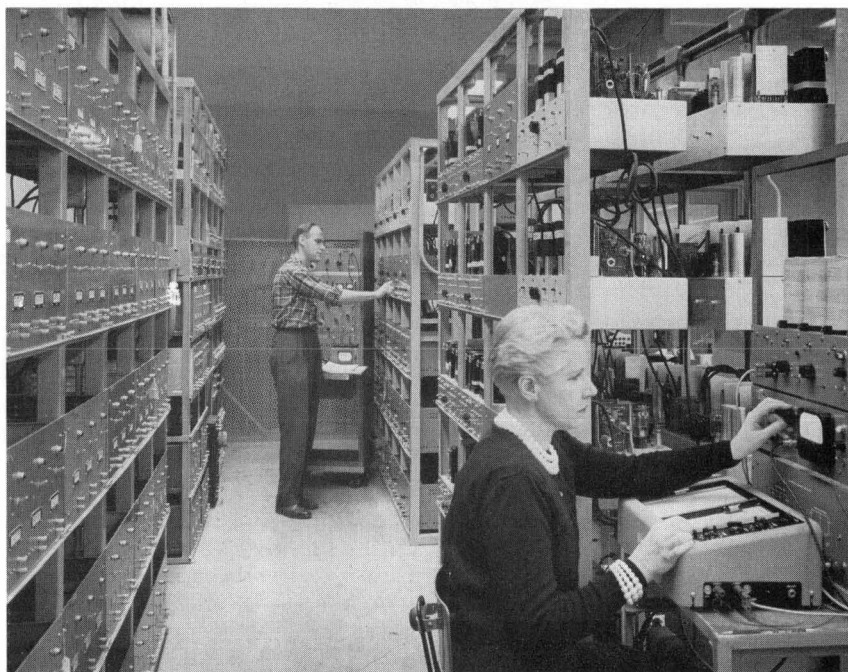
Daily measurements of crystal frequency are made and recorded while plate is continuously operated in test stands for several-week period. Before aging, crystal temperature characteristic is plotted with automatic set-up (foreground) and proper oven temperature determined.
